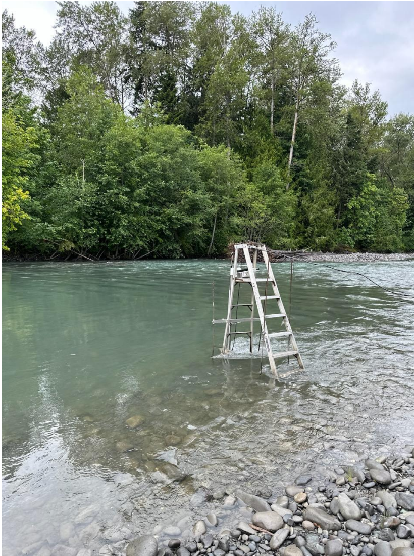
Figure 2. Looking downstream at the lower SONAR site, labeled “Old OM Sonar Site” in Figure 1. The SONAR is attached to the pole mount which is in turn attached to the ladder. The SONAR recorded data at this site from September 2 through October 20, 2025.
