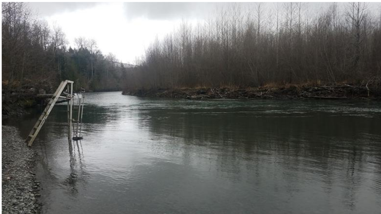
Figure 3. Upper SONAR site looking upstream. This site is labeled as “New OM Sonar Site” in Figure 1. The SONAR is attached to the pole mount which is in turn attached to the ladder. The SONAR recorded data at this site from October 20 through November 26, 2025.
